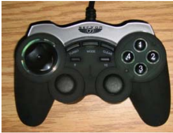
Figure 13. Xtreme Gaming Sector 7 game controller. Physical input uses the four thumb-operated buttons on the right-hand side.
